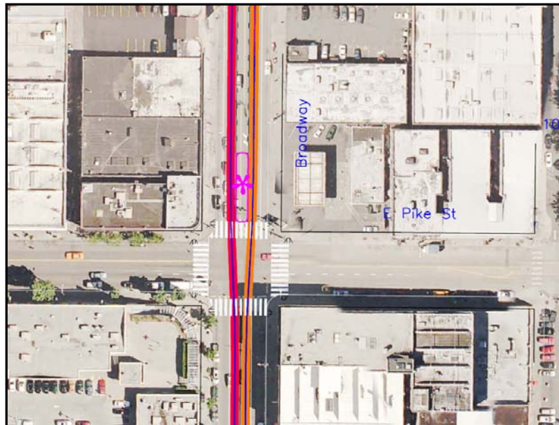
Figure 3 - Center Lane/Center Platform on Broadway Ave at E Pike Street
